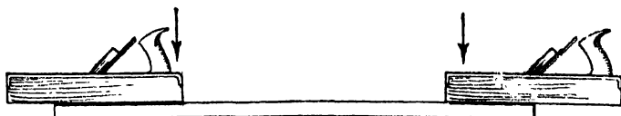
FIG. 16.—WHERE PRESSURE IS APPLIED WHEN PLANING.
